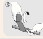
Pull the tape until the width of the tape is reduce by around <u>2~3mm</u> and wrap it around the cable.
