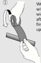
Wrap around the cable with the tape in half width overlapping, and after completing the first layer, apply the upper layer.
