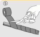
Cut the tape. It is recommended to stabilize the wrapped tape by applying a plastic tape.
