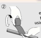
To make your work easier, it is recommend to stabilize the tape by using a plastic tape at the beginning of the wrapping point.
