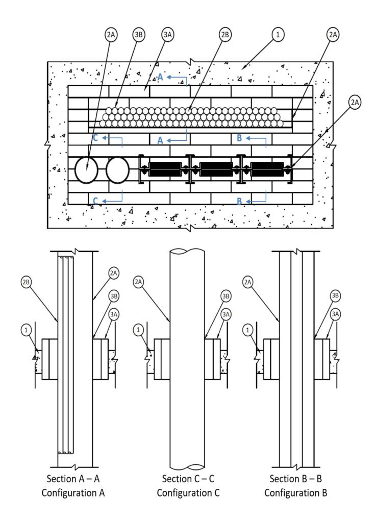
1. **Floor or Wall Assembly** — Min 114 mm (4-1/2 in.) thick reinforced normal weight (2320-2480 kg/m<sup>3</sup> or 145-155 pcf) concrete. Wall may also be constructed of any UL Classified Concrete Blocks<sup>\*</sup>. Max area of opening is 0.6 m<sup>2</sup> (930 in.<sup>2</sup>) with a max dimension of 1200 mm (47-1/4 in.).
